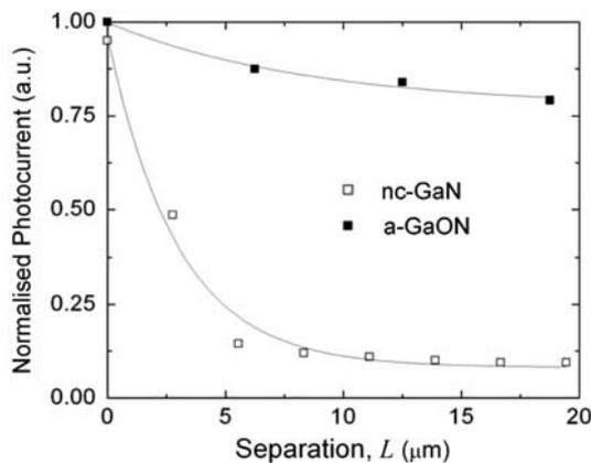
**Fig. 2** Photocurrent versus separation between edge of laser spot and contact. The solid lines are guides for the eyes
