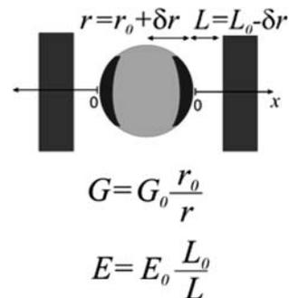
**Fig. 3** Schematic of the laser spot between contacts, and determination of generation rate and electric field dependence on spot size
