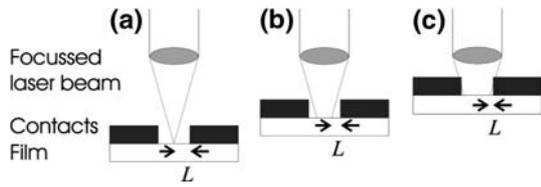
**Fig. 1** Schematic diagram showing how  $L$ , the separation between the laser spot and electrodes changes as the film is moved through the focussing cone of the laser beam
