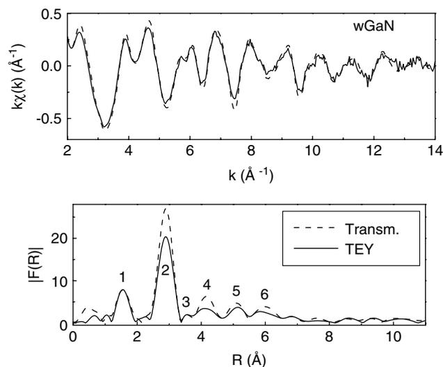
**Figure 1.** Comparison of EXAFS spectra of the polycrystalline wGaN recorded in transmission (dashed line) and TEY (solid line) mode (top) and modulus of the corresponding pseudo radial distribution function (bottom).
