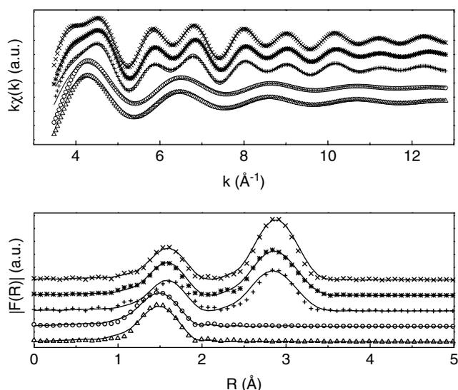
**Figure 6.** Comparison of experimental (symbols) and simulated (solid lines) modulus of the pseudo radial distribution function (not corrected for phase shift) of the first shell of GaN10 and GaN28 and the first and second shells of GaN30, GaN40, GaN80 and wGaN.
