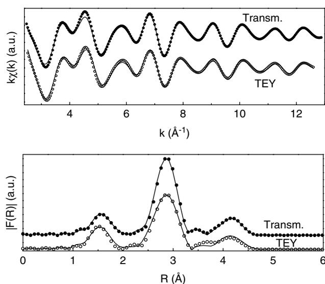
**Figure 2.** Fourth-shell filtered EXAFS (top) and modulus of the pseudo radial distribution function (bottom) extracted from transmission and TEY wGaN spectra. Comparison of experimental (symbols) and simulated (solid lines) data.
