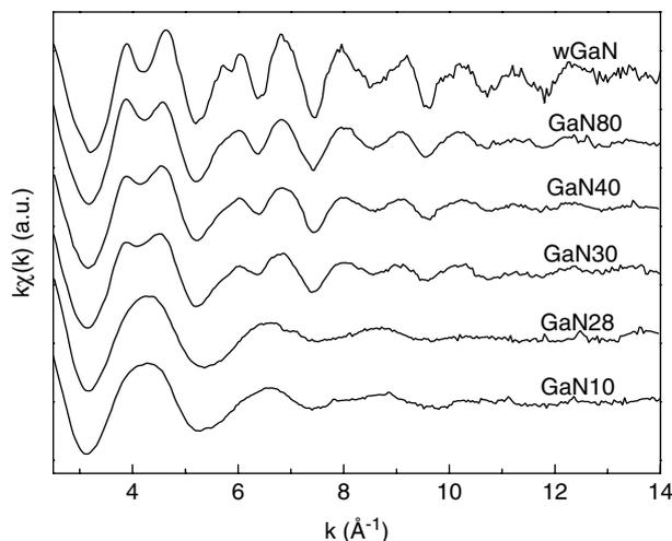
**Figure 4.** The EXAFS oscillations extracted from TEY x-ray absorption spectra of GaN10, GaN28, GaN30, GaN40, GaN80 and wGaN.
