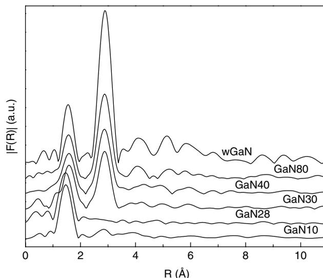
**Figure 5.** Modulus of the pseudo radial distribution function ( $|F(R)|$ ) (not corrected for phase shift) of GaN10, GaN28, GaN30, GaN40, GaN80 and wGaN, from bottom to top.
