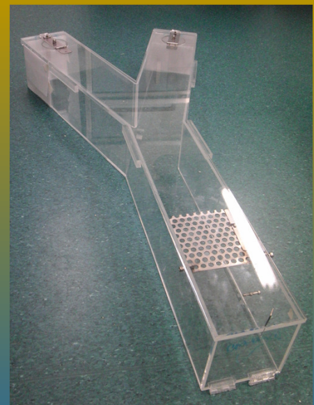
Figure 3: Y-maze used to test potential attractants for rats
