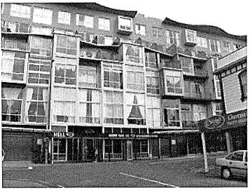
Where setbacks are created that run parallel to the prevailing wind however, the effect is lost as it effectively becomes a wind channel at ground level. It is generally recommended that set backs are a minimum depth of 3m or there will be little effect on the wind.
