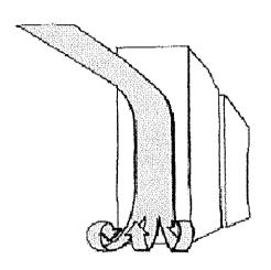
rectangular buildings, is that the windward face should be kept as small as possible. The larger the area of the exposed windward face, the more downwash is induced. So tall, wide buildings should be designed with their wide face parallel to the prevailing winds, and their narrower faces exposed – perpendicular to the prevailing wind direction Generally it is accepted that the following is true for wind and height;
