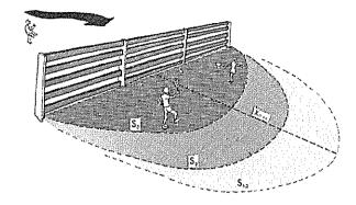
The final formula required for this allows the downwind length of the shelter to be worked out.
