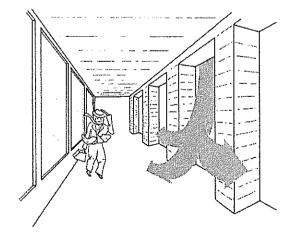
When there are low and high buildings next to each other, due to the low and high effect the space in between has high discomfort effects, it is possible to roof over between the buildings to increase discomfort levels.
