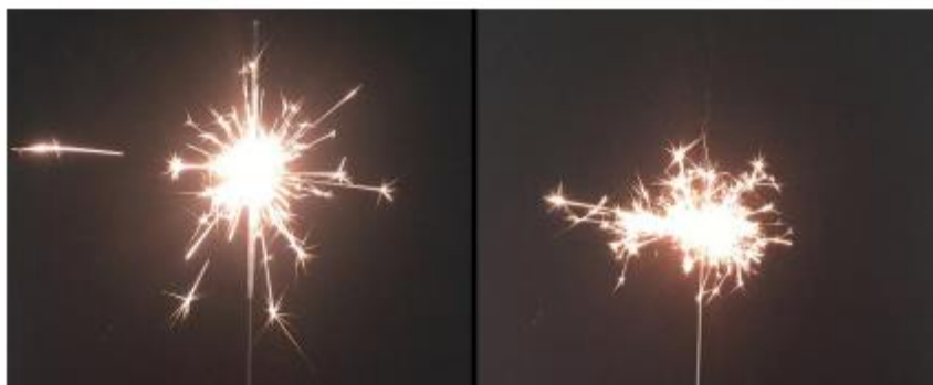
Figure 6: Spark pattern of a self-made sparkler (left) and a bought sparkler (right).
